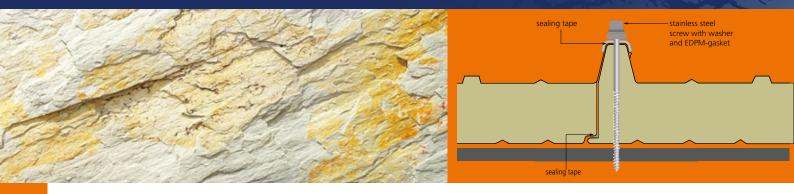
This sandwich panel with non-combustible insulation core made of rock wool meets today's high demands for fire protection. According to the guidelines for industrial construction, non-combustible insulation materials are obligatory, particularly for large-surface and multi-storey buildings. For core thickness of 100 mm and higher a fire resistance up to 90 minutes can be reached. Additionally Hipertec® Roof panels show exceptional acoustic
